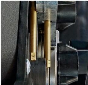
**Ultra-low drag inlet guide pins** make loading the wire easy and do not deform the wire on the way into the drive rolls. Simply thread the wire through the pins and into drive rolls. There are two ways to advance the wire through the drive roll and into the gun. Either open the pressure arm and thread the wire into the grooves in the drive roll and on into the gun inlet **or** place the wire between the pins and use the jog/purge switch to advance the wire through the drive roll.
