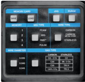
**Internal control panel** duplicates many front panel selections so the processes can be configured and selected from the front panel while using, or from the inside while loading wire and preparing the Smart Feeder for use.
