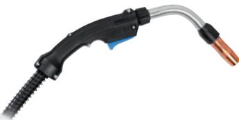
Recommended for root pass welding, especially in fixed-position applications where visibility is difficult. Comes with 15-foot (4.6 m) cable, tapered tip and nozzle. NEMA rated at 350 amps at 100 percent duty cycle with CO<sub>2</sub> gas. Switch to a standard tip and nozzle for fill and cap pass welding with flux-cored or pulsed MIG welding processes. This allows one gas and one wire to make the weld.
