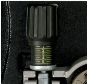
**Scaled wire pressure knob** provides easy adjustment and consistent pressure on the drive rolls and wire. **Wire drive and motor assembly** is specifically designed for mobile welding applications to provide smooth and consistent wire delivery. Improved motor torque and drive roll system are designed to feed small-diameter solid wire (.023 inch) to large-diameter cored wire (5/64 inch).
