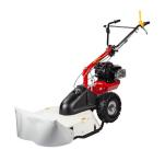
Rotor: single Cutting: 6 pivoting blades Working width: 63 cm Cutting height: 5 o 8 cm
