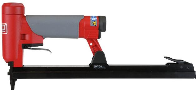
Xtreme Quality for industrial light wire stapling this durable, fine-wire Senco air powered tool is designed for professional performance. Various SFT10XP models drive staples ranging in length from 5mm to 16mm and has excellent features for user comfort, with a double length magazine reducing down time increased productivity
