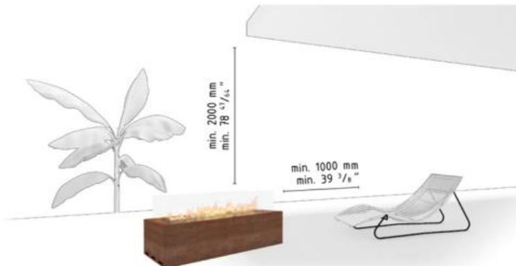
*Fig. 1: Minimum distance to flammable materials*
