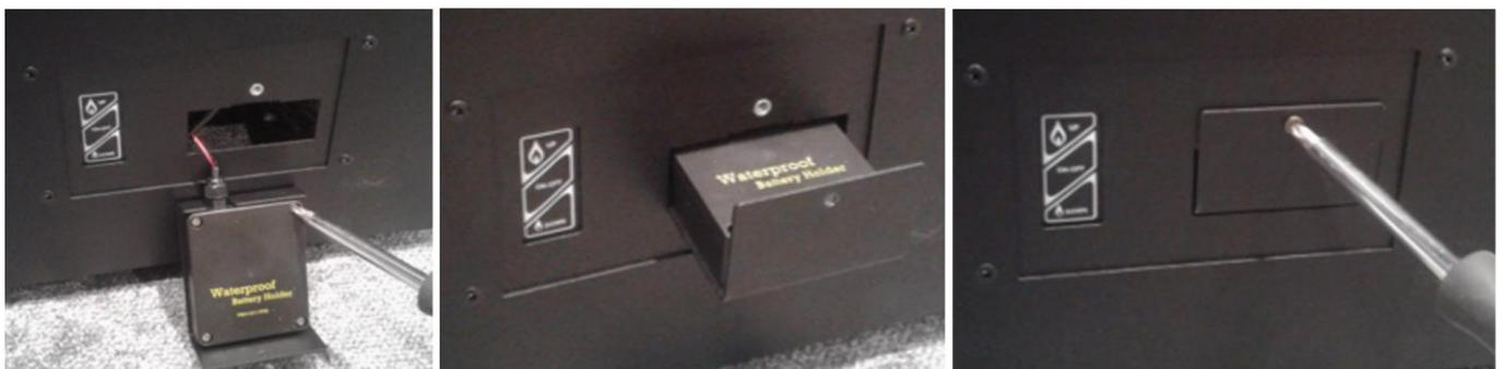
*Fig. 11 – Putting back the battery box*
