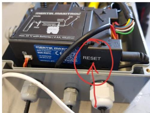
Fig. 7 – Receiver “RESET” button
