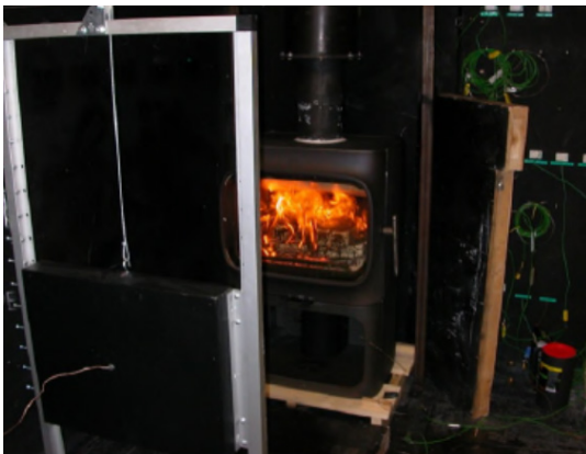
The stove on the test rig, safety test
