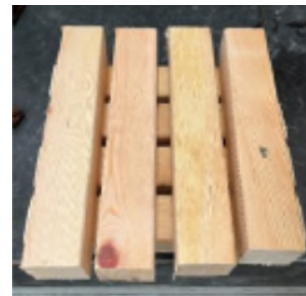
Placement of the fuel load in the firebox
