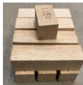
Placement of the fuel load in the firebox
