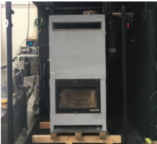
The stove on the test rig, output test
