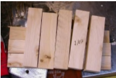
Placement of the fuel load in the firebox
