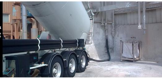
Bulk tank truck discharge
