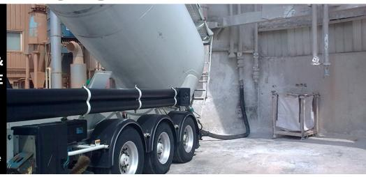
Bulk tank truck/Suction and discharge
