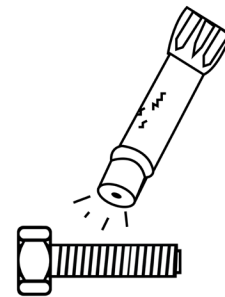
Figure 2. Apply Ant-Seize to Bolts
