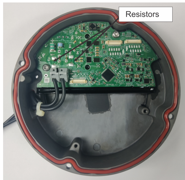
Figure 9: 1-connector converter (2 fuse resistors)
