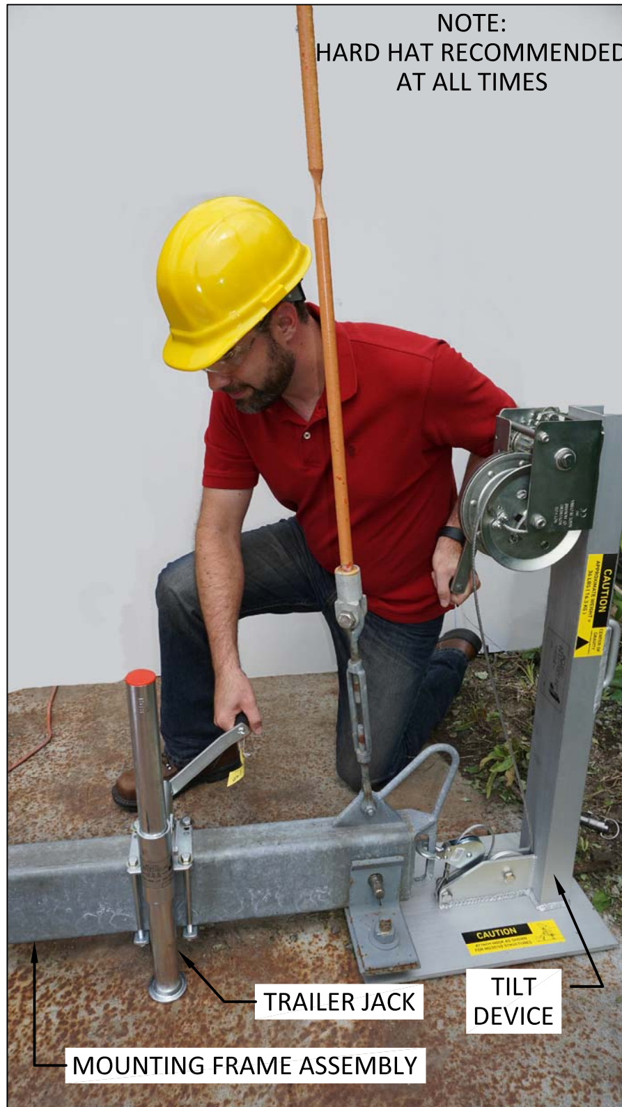
FIGURE 3-5 LOWERING MG-30/40 STRUCTURE (Ref. Section 3.3)
