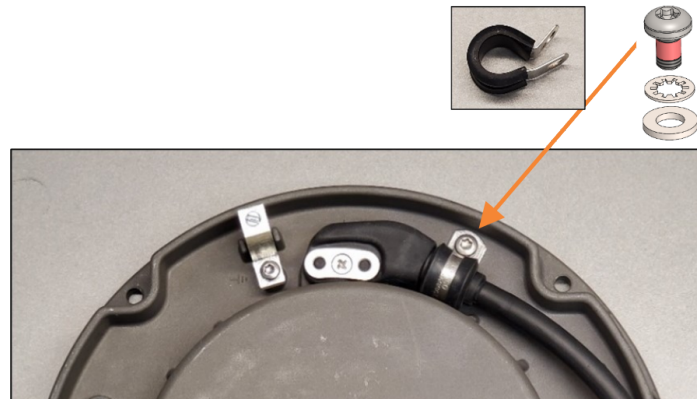
Figure 26: Cable clamp, bolt, washer and lock washer
