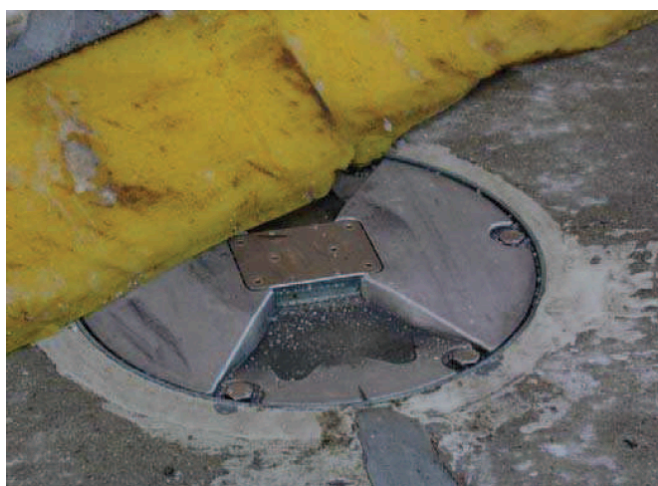
Figure 61: Signs of wear on plastic cutting edge
