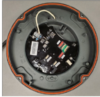
Bottom pan with installed gasket, 12-inch
