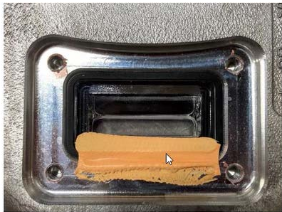
Figure 14: Removal of Deformed Orange Thermal Pad
