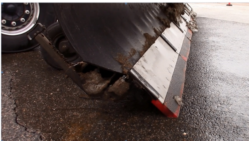
Figure 39: Fig. 1 — Snowplow blade with well aligned segments
