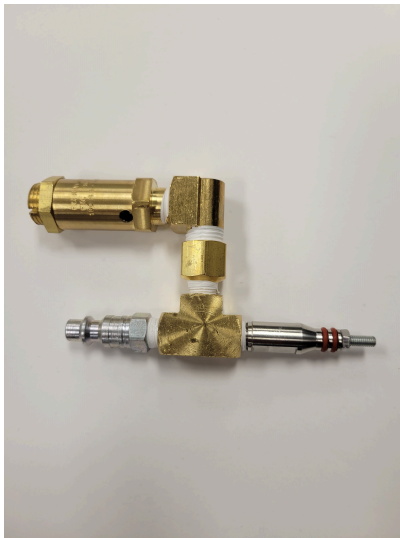
Figure 25: Pressure test fitting tool
