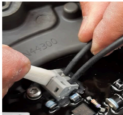
Figure 43: Releasing/locking secondary wires with insert tool
