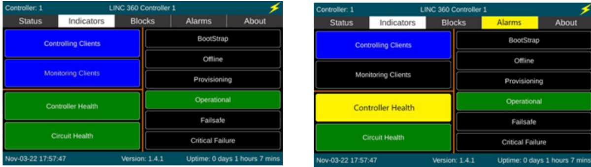
Figure 13: Left: Indicators with Alarms. Right: Indicators with Circuit Alarms
