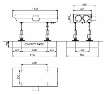
**Note:** Dimensions of concrete block are given for information and must be review according of the site
