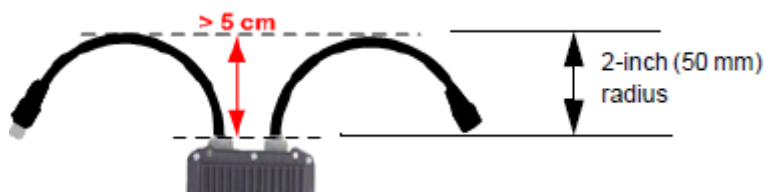
Figure 9: Remote Max. Bending Radius
