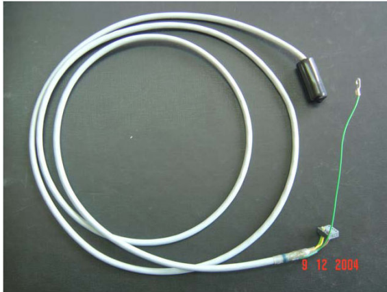
Figure 44: External Temperature Probe (1440.21.000)
