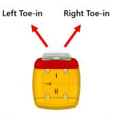
Toe-in determined by standing on top of the light fixture looking in the direction of the beam.
