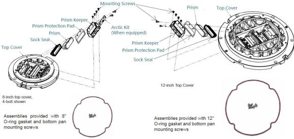
Figure 62: Bottom Pan Assembly, 8-inch
