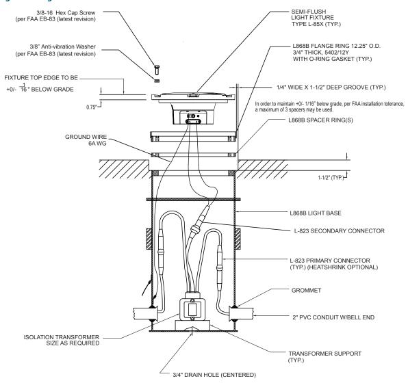
1. Torque according to: FAA EB-83 (latest revision).
