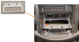
11. Install the Prism-keeper Plate into the top cover with 2 M4x10 screws (26 in-lbs/3 Nm) to the "top" of the Prism-keeper
