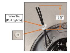
13. Tighten the new Cord-set-retainer Bolt at 26 in-lbs (3 Nm).
