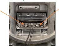
12. Finish the mounting procedure for the Prism-keeper Plate with 4 M4x8 screws at 26 in-lbs (3 Nm) to the "bottom" of the prism keeper plate.
