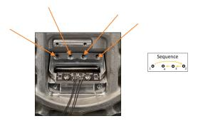
13. Mount the Light Engine Assembly onto the top cover with 4 new M4x10 screws at 26 in-lbs (3 Nm).
