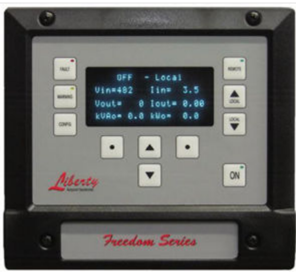
Figure 10: Operator Interface Display
