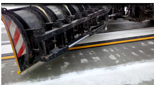
Figure 79: Snowplow without support wheels
