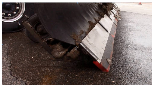
Figure 75: Snowplow blade with well aligned segments
