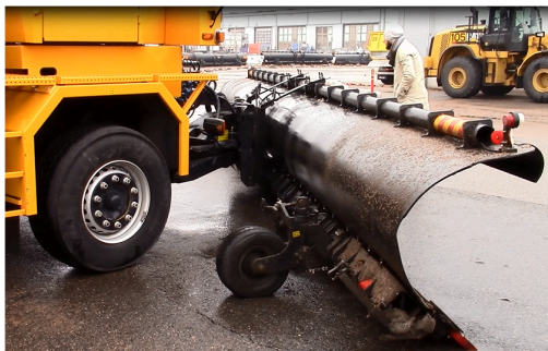
Figure 78: Snowplow with support wheels
