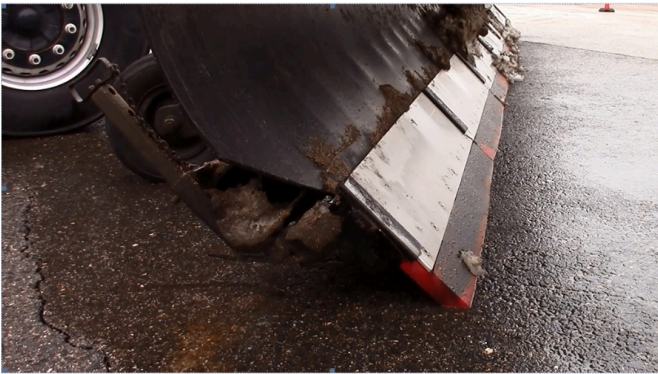
Figure 1. Well-aligned plastic cutting edge
