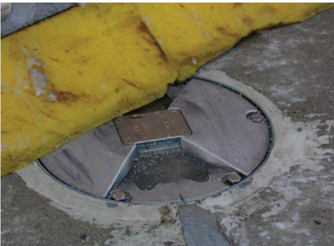
Figure 2. Signs of wear on plastic cutting edge
