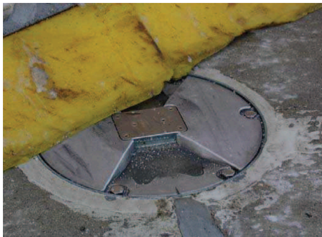
Figure 72: Signs of wear on plastic cutting edge
