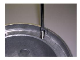
2. Remove old Loctite residues using a thread-cleaning device, size
