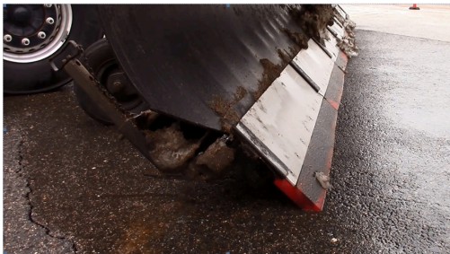
Figure 38: Snowplow blade with well aligned segments
