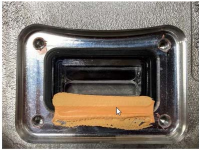
Figure 17: Removal of Deformed Orange Thermal Pad
