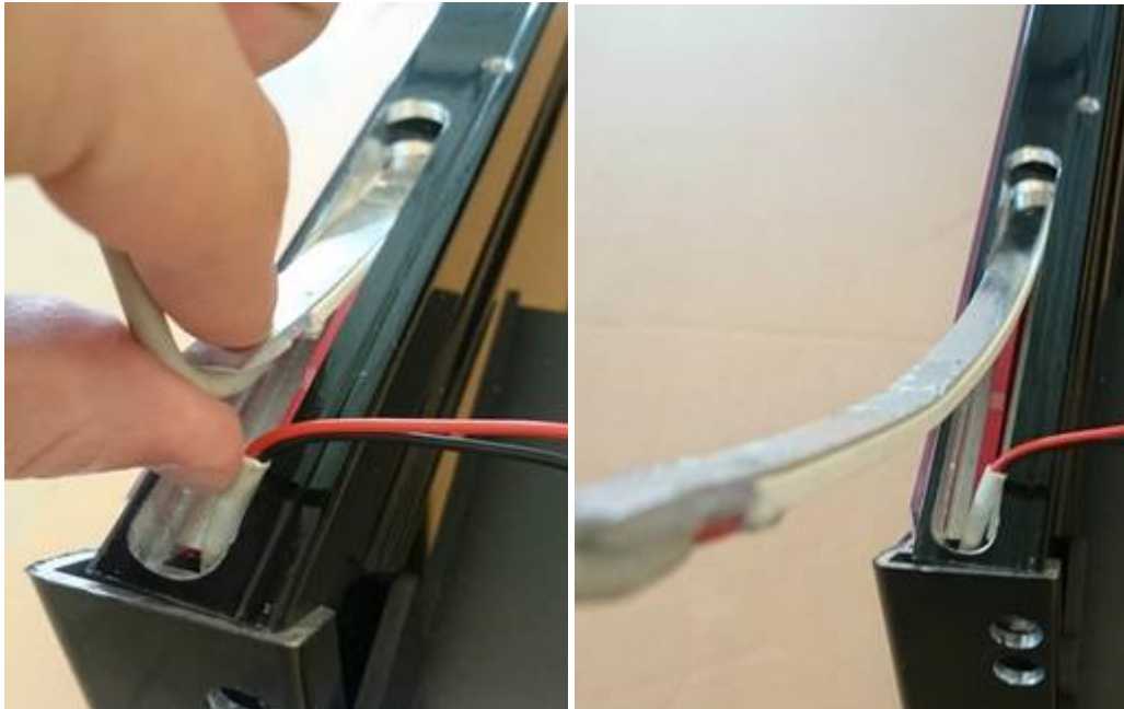
Figure 24: Pull out LED-strip
