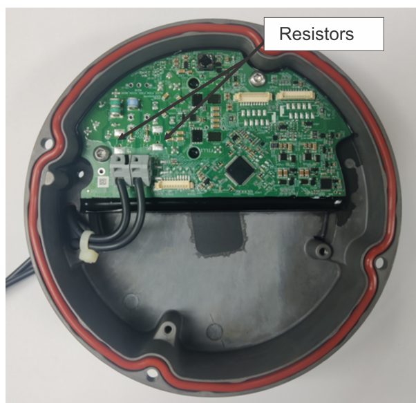
Figure 11: 1-connector converter (2 fuse resistors)
