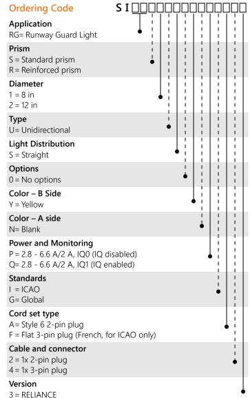
**Note:** The IQ - functionality allows control and monitoring of the RELIANCE IQ. IQ1 fittings are pre - configured for the specific position at delivery. IQ 0 fixtures needs to be configured before use.
