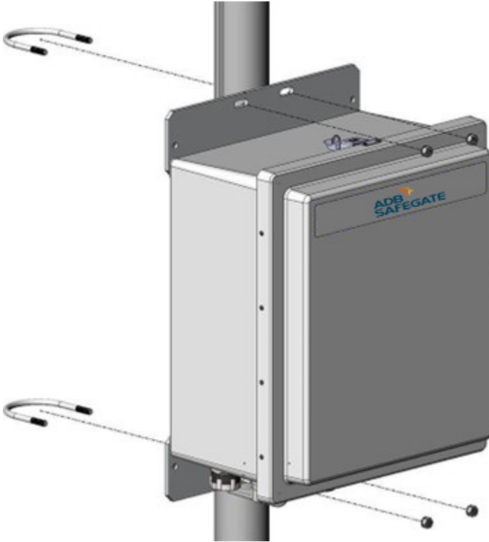
Figure 13. Electronics Enclosure Mounting
