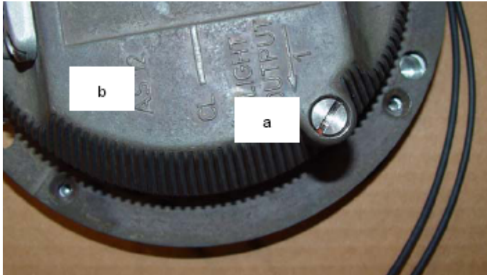
Figure 11: Removing Pressure Release Screw
