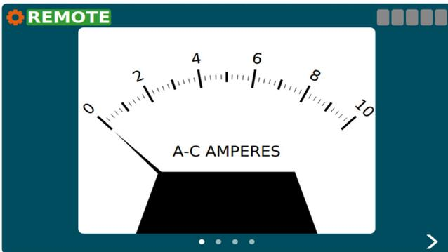
This view is shown when the ACE3 mode is "CCR" and the display mode is L828 or when the "Display Analog Current Gauge" feature is enabled.
