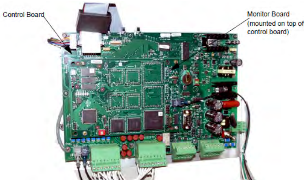
Figure 7: ACE Control and Monitor Boards
