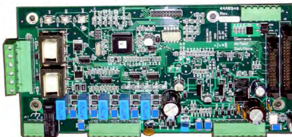
Figure 6: CCT Control PCB (44A6546)
