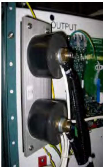
Figure 35: Output Lightning Arrestors
