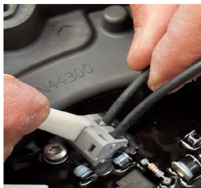
Figure 26: Releasing/locking secondary wires with insert tool
