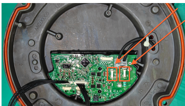
Figure 10: 1-connector converter (2 fuse resistors)
