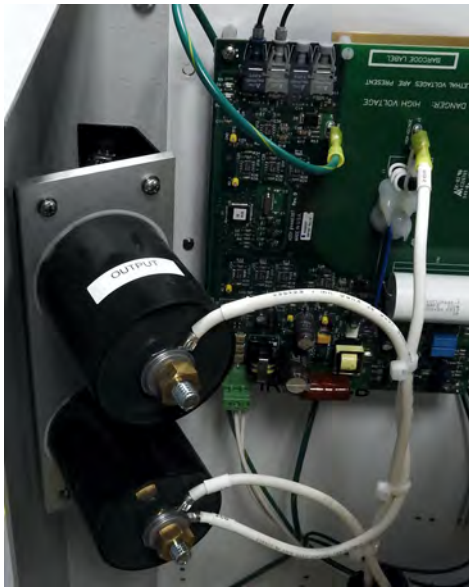
Figure 50: 94A0576 Type Output Lightning Arrestors
