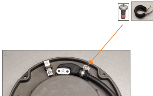
Figure 30: Dispose Old Bolt, Washer and Lock Washer
