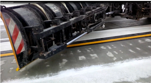
Figure 69: Snowplow without support wheels
