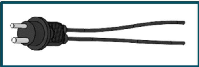
Figure 26: Style-6 Secondary Cable
