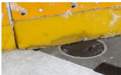
Figure 67: Snowplow blade without clearance
