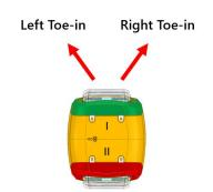
Toe-in determined by standing on top of the light fixture looking in the direction of the Threshold beam.
