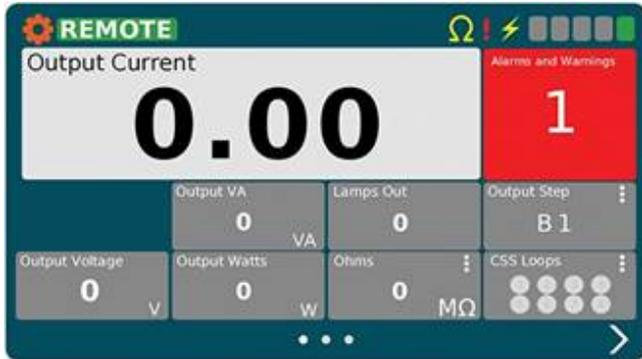
The ACE3 unit provides L-829 monitoring and optional megging or CCR input monitoring capability. Each unit is installed locally at each CCR that requires remote control and/or monitoring within the airfield lighting electrical vault. Optional CCR input monitoring monitors the following:
