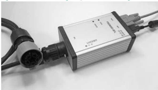
Figure 14: Parameterizing adapter for the settings of an inset flashing light
