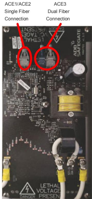
The CVM2 is the latest generation monitoring module. This module is backward compatible with all previous versions of CVMs and can be used as a direct replacement.
