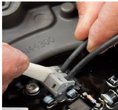
Figure 42: Releasing/locking secondary wires with insert tool
