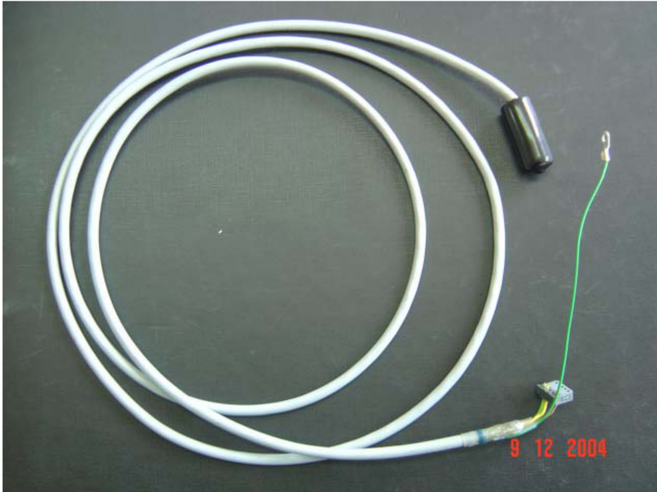
Figure 45: External Temperature Probe (1440.21.000)
