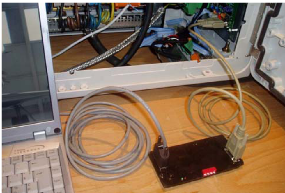
Figure 46: Connection: ICC, Dongle and Laptop
