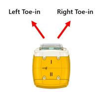
Toe-in determined by standing on top of the light fixture looking in the direction of the beam.
